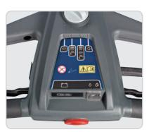
The SC350 offers four operating modes, including: off, water + brush, water + brush + vacuum, and vacuum only. Two adjustable flow rates—low and high—allow operators to easily match diverse application requirements.
